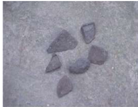
Photo 5 – Old Train Block Fragments containing Asbestos
