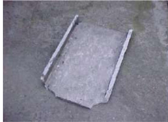
Photo 2 – Moulded Asbestos Cement product – Cable Tray
